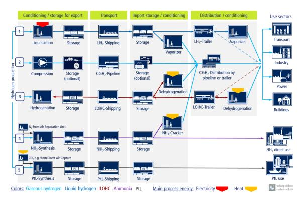
Figure 23:Main elements of large-scale hydrogen export/import supply<br/>chains (1) LH2 via ship, (2) CGH2 via pipeline, (3) LOHC via ship,<br/>(4) NH3 via ship, and the supply of PtL for comparison (5)
