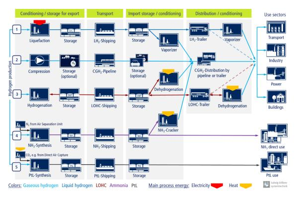
Figure 23: Main elements of large-scale hydrogen export/import supply chains (1) LH<sub>2</sub> via ship, (2) CGH<sub>2</sub> via pipeline, (3) LOHC via ship, (4) NH<sub>3</sub> via ship, and the supply of PtL for comparison (5)
