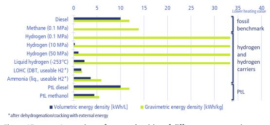
Figure 17: Comparison of energy densities of different energy carriers
