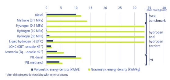
Figure 22: Comparison of energy densities of different energy carriers
