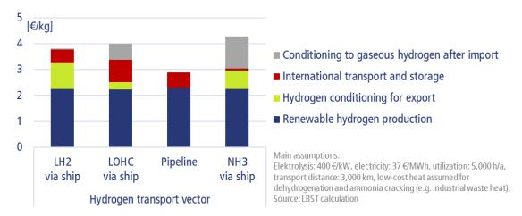
Figure 25: Main cost elements of large-scale hydrogen import in €/kg<sub>H2</sub>
